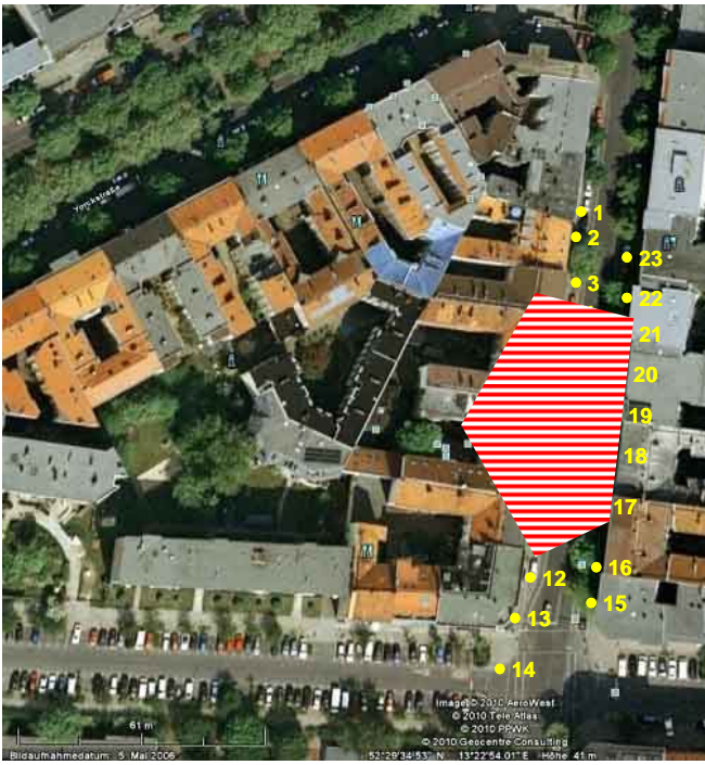
Figure 7. Coverage IEEE802.15.4-2006 PSSS 868MHz "TRx154b_Eval" module 0 dBm Tx power and 250 kbps data rate. Map source Google Earth.
