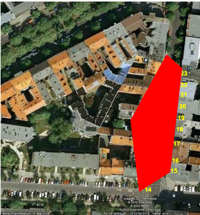
Figure 8. Coverage IEEE802.15.4-2006 PSSS 868MHz "TRx154b_Eval" module 10 dBm Tx power and 250 kbps data rate. Map source Google Earth.
